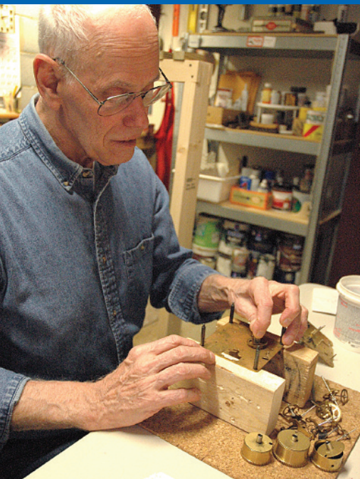
LEFT: Richard replaces a brass bushing, a tiny pin-like piece that is a vital part of the bearings of mechanical time-tellers.
